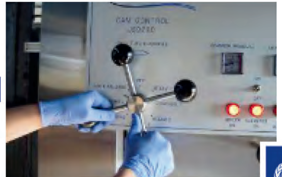
Start heating , multi-vacuum and sterilization cycle.
