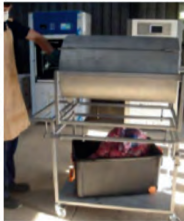
Unlock and rotate the barrel to dump treated waste at the bottom
