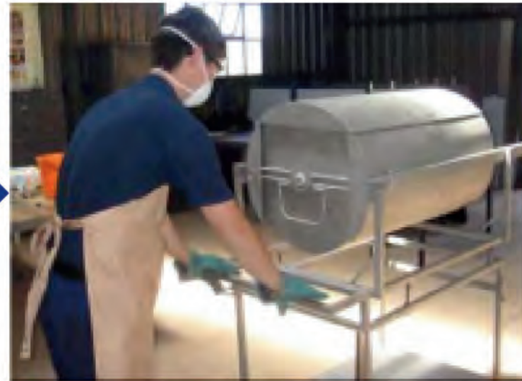
When barrel is full, move to autoclave
