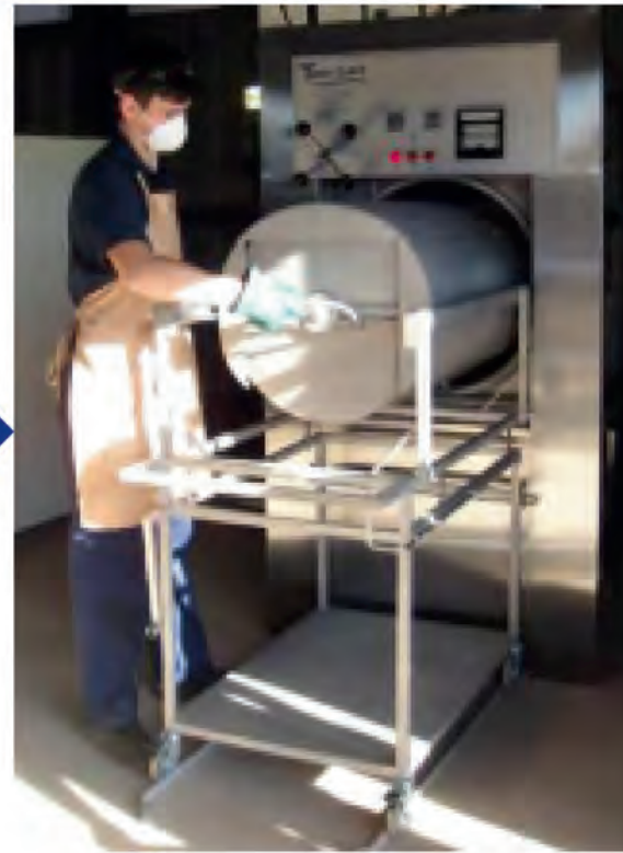
Slide barrel into Autoclave
