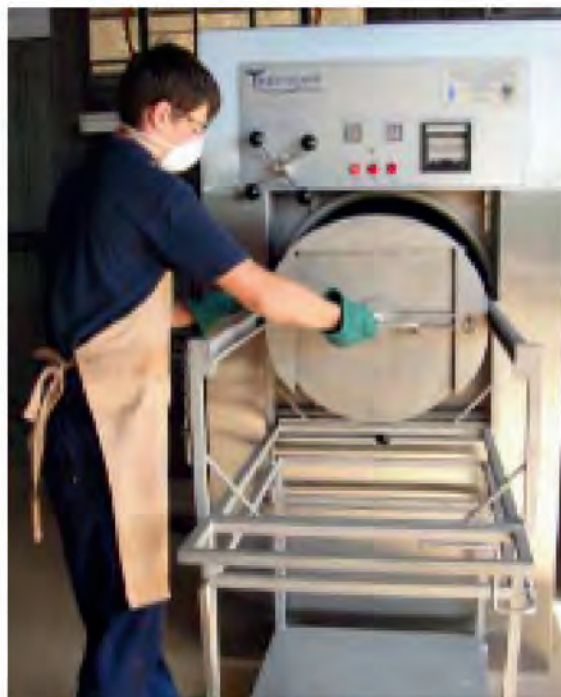
When finished open the door and remove the sterilized barrel
